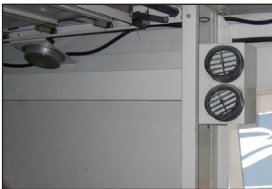
Mounted intake fan forces outside air to the front of the vehicle.
